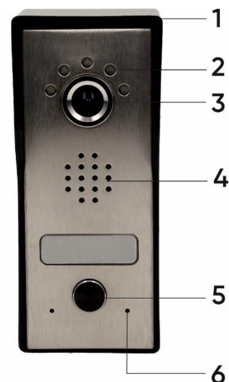
fig. 2 Construction of the outdoor unit
