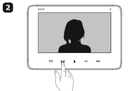
To open the outside gate, press the GATE CONTROL button.
