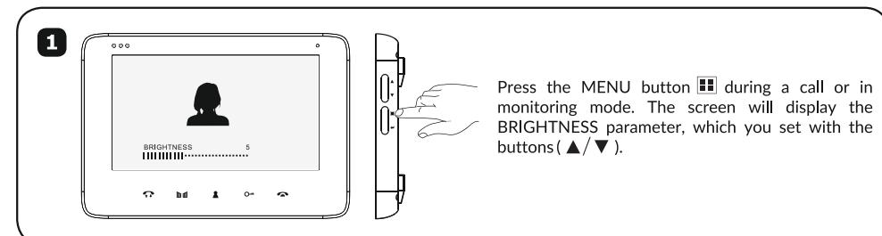
Press the MENU button during a call or in monitoring mode. The screen will display the BRIGHTNESS parameter, which you set with the buttons ( $\Delta/\nabla$ ).
