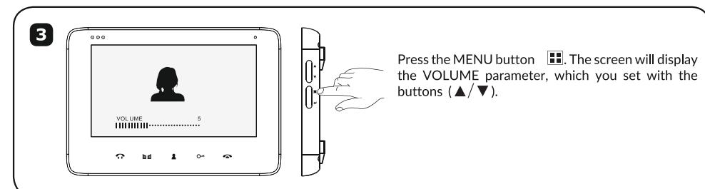
Press the MENU button . The screen will display the VOLUME parameter, which you set with the buttons ( $\Delta/\nabla$ ).
