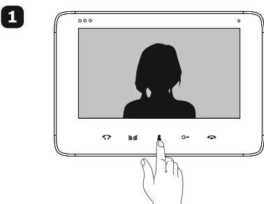
To preview the camera image, press the MONITORING button. Press the same button again to return to standby mode.
