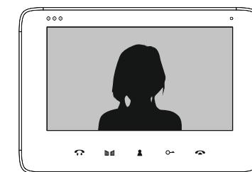
The internal monitor will activate the ringing tone and the external camera image will be displayed on its screen
