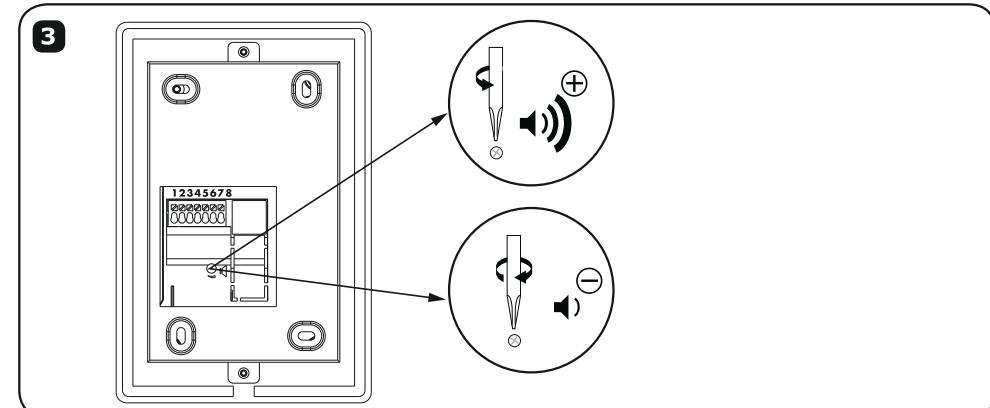
4. Connect the wires according to the wiring diagram (see point 5) and set the volume level for the outdoor cassette.
