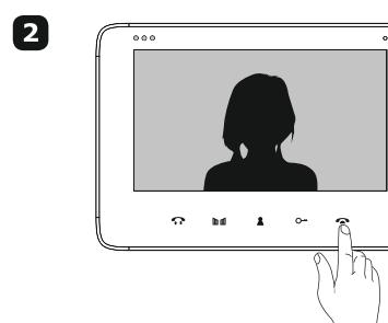
Press the TALK button to start a conversation with the person standing outside. Press the same button again to turn off the monitor panel.
