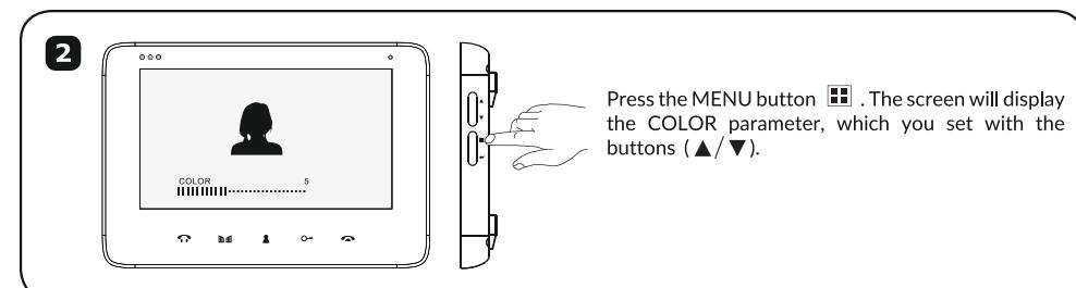
Press the MENU button . The screen will display the COLOR parameter, which you set with the buttons ( $\Delta/\nabla$ ).
